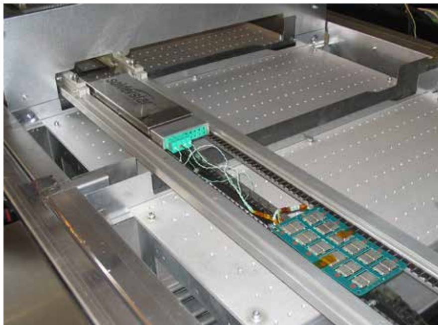
■ Figure 1. A profiler with four thermocouples attached to crucial components.
