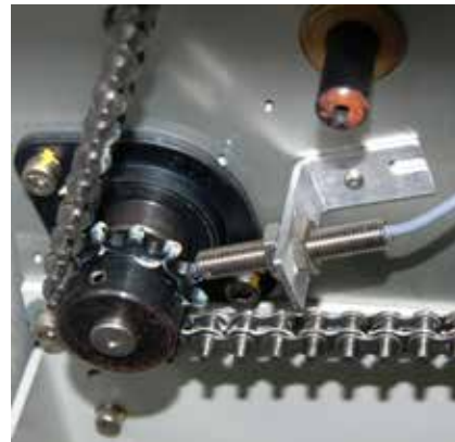
■ Figure 5. Close up of the speed sensor monitoring the conveyor speed.
